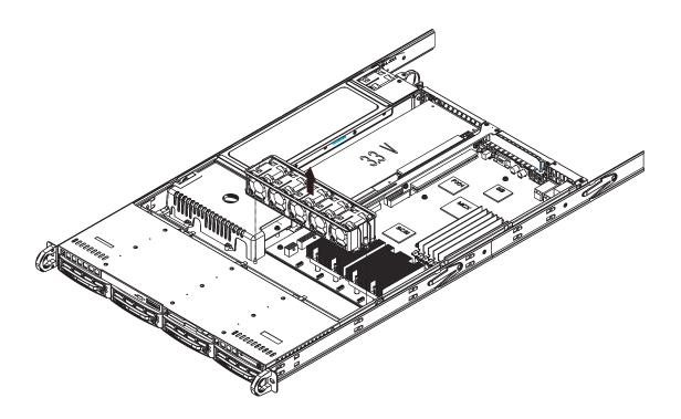
Figure 6-2. Removing the Fan Housing
